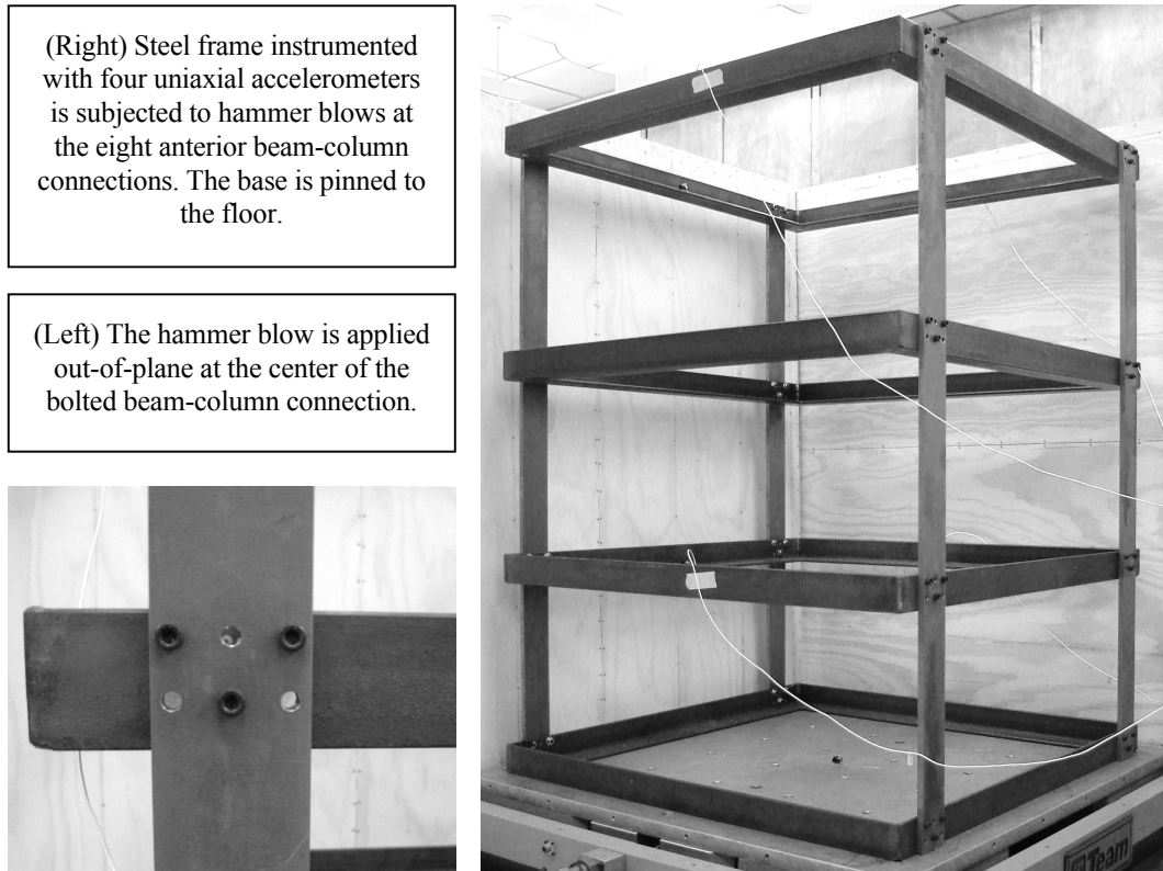
Figure 1. Instrumented steel frame (right) and beam-column connection (left).
