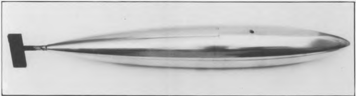
(b) Hull shape after plating
