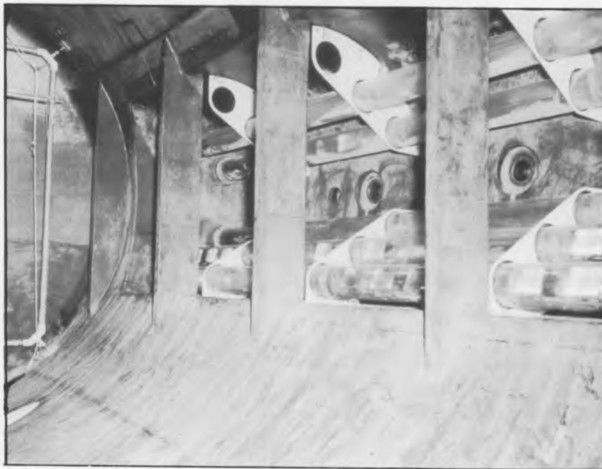
(a) Tank bulge after draining
