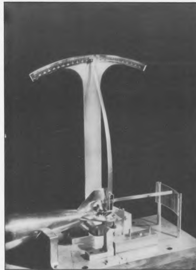
(c) Stern plane and rudder angle measuring setup for Albacore model (vertical maneuvers)
