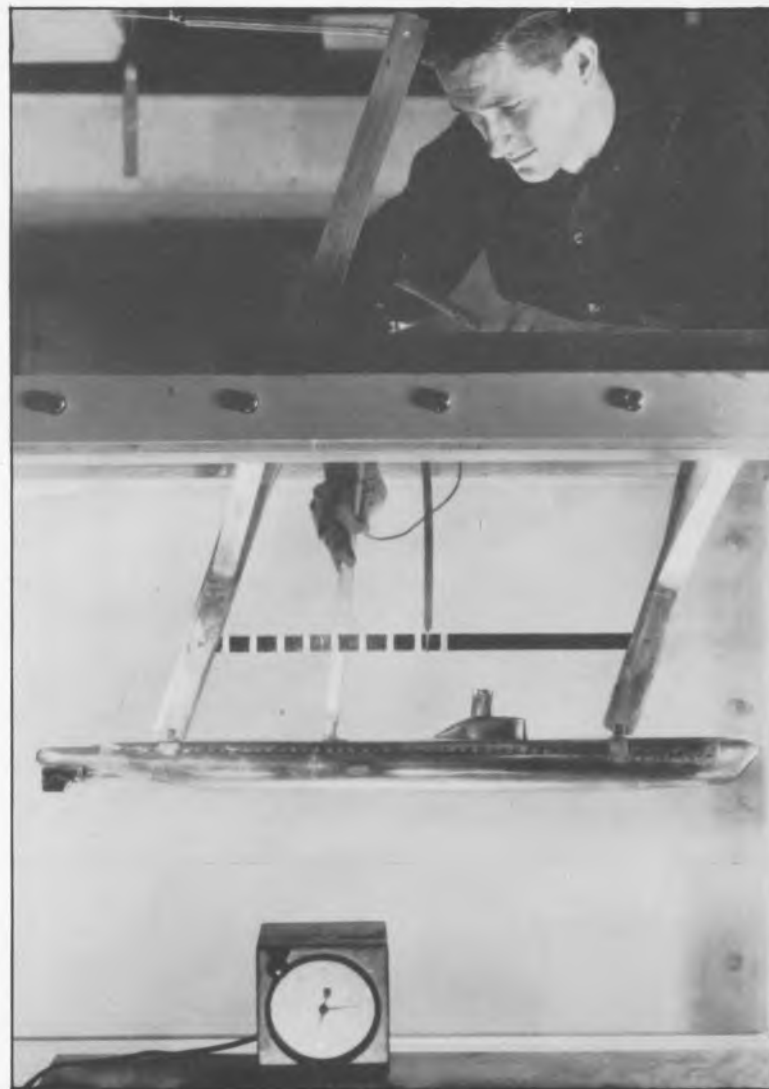
(b) Model mounted on free swinging parallelogram support
